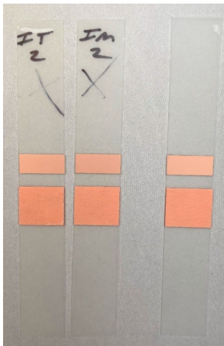
Picture #4 Results for Aborted Instrument cycle shown with unused strip on the right
