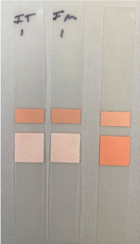
Picture #5 – Instrument cycle – complete cycle shown with unused strip on the right PASS results shown, Indicator pad is lighter in color than reference pad.
